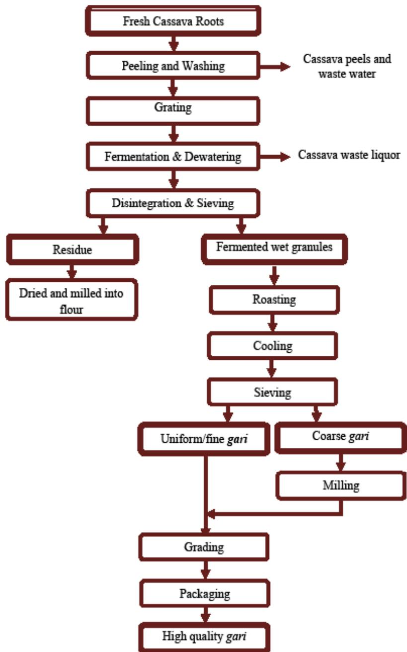
Figure 1. Flow chart for the production of *gari*.
